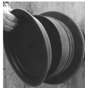
4. Place second end cap on sleeve. Check to determine that the cap is properly inserted.
